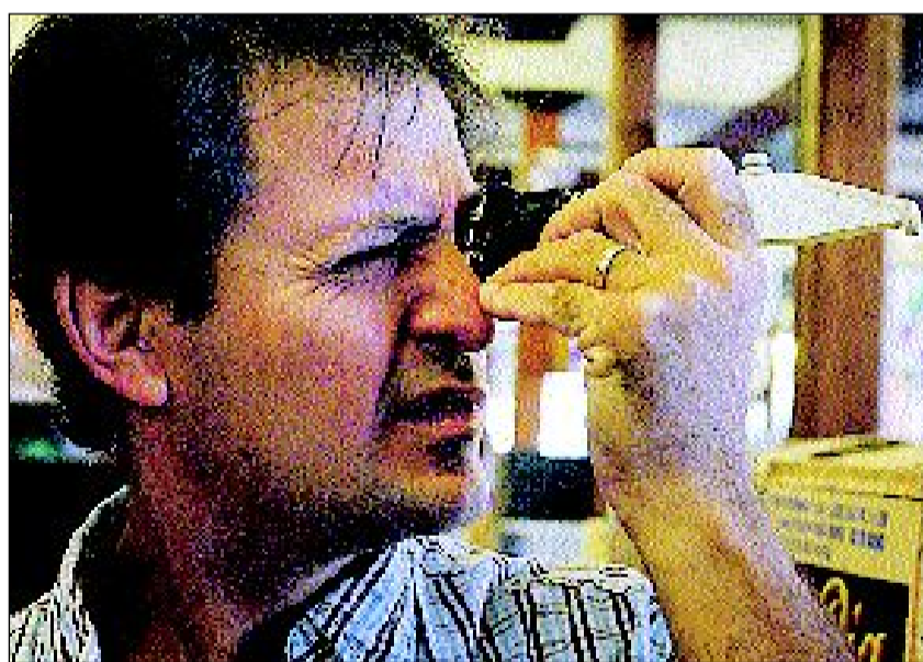
Soterios Georghiou of Ringwood uses a refractometer to measure the brix (sugar content) of grapes at Corrado's.
